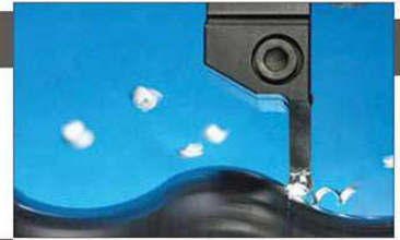
• MRGN type : Full "Round" geometry
